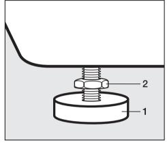
■ Hold the foot 1 firm using a pipe wrench and using a spanner turn the counternut 2 to the right firmly up against the housing.
